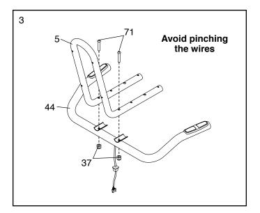
Have a second person hold the Seat Handlebar (44) near the top of the Rear Frame (43) until step 5 is completed.
